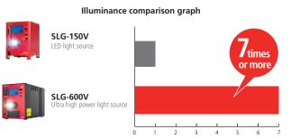
\*Measured value at an each given distance from the fiber exit face of 1,000 mm long straight light guide (with 8 mm bundle diameter) at maximum illuminance ( not guaranteed )
