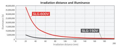
\*Measured value at an each given distance from the fiber exit face of 1,000 mm long straight light guide (with 8 mm bundle diameter) at maximum illuminance ( not guaranteed )
