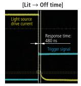
Strobe lighting in accordance with external trigger signals
