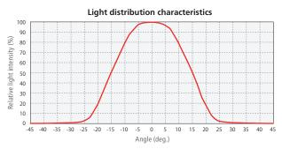
\*Measured value at an each given distance from the fiber exit face of 1,000 mm long straight light guide (with 8 mm bundle diameter) at maximum illuminance ( not guaranteed )
