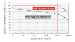
\*The graph is an image when the stabilization time is set to 10,000 hours. (not guaranteed)
